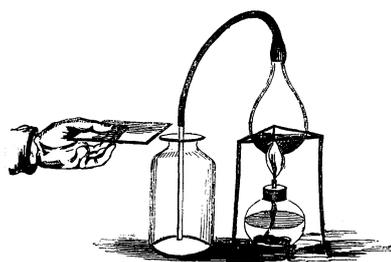
much as this liquid absorbs it with great rapidity. It must be collected over mercury, or by displacement. The latter process serves well enough for all ordinary occasions, and the complete method of conducting the operation is represented in the annexed woodcut.
