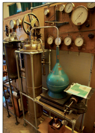
▲ The museum-kept nitrogen and oxygen liquefier of Kapitsa
