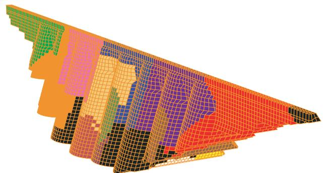
Figure 1: Finite element mesh of a buttress dam used to evaluate the structural response to earthquakes. The mesh is distributed across processors as illustrated by the colouring.
