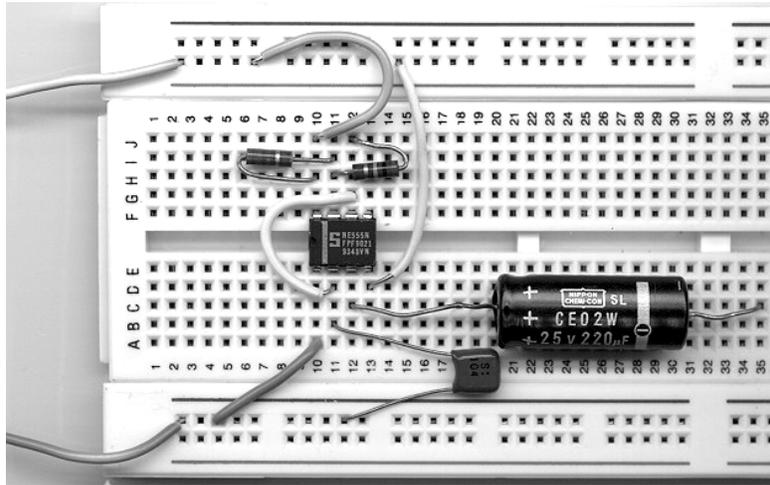
Figure 1 Oscillator circuit using 555 I.C.
