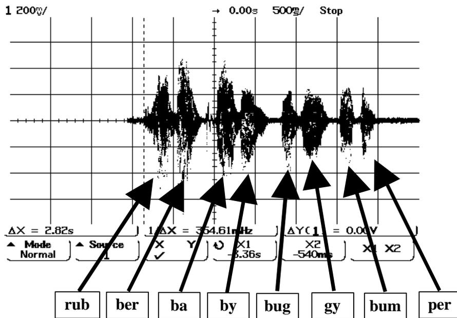
Figure 4 Digital Oscilloscope Envelope Display of Voice
