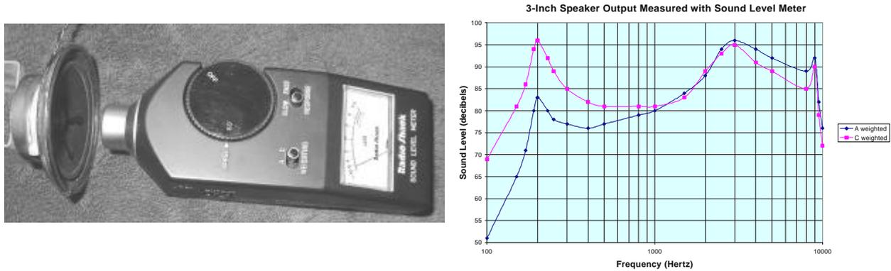
Figure 3 Sound-Level Meter (left), Frequency Response of 3-Inch Speaker (right)
