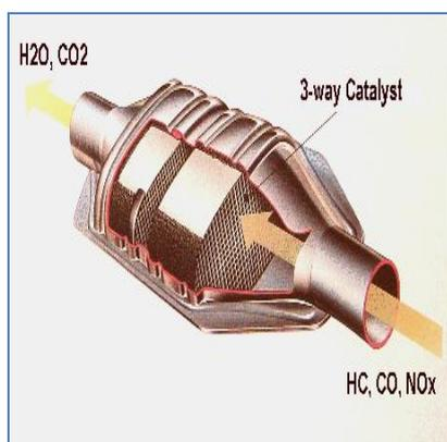
**Fig. 11. Ceramic honeycomb and catalytic converters.**
