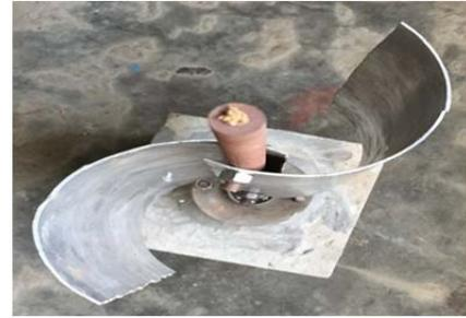
**Fig. 2: Fabricated Two-bladed Savonius Rotor.**
