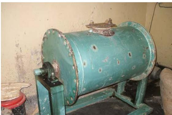
Fig 3: Ball Mill, is an equipment that has increased in quality clay production and reduced wastage
