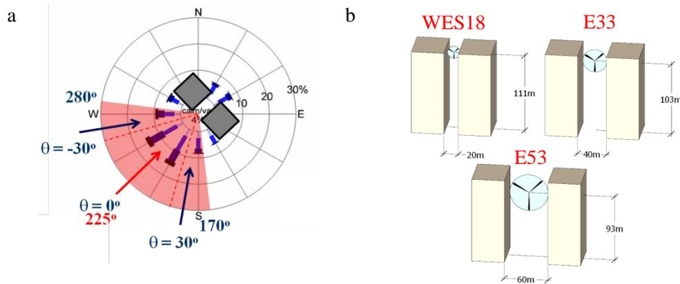
Figure 3: (a) Orientation of buildings in prevailing wind direction based on annual wind rose (top view); (b) Positioning of wind turbines depending on passage width
