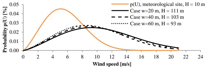
Figure 4: Modified wind PDFs for passage widths of 20m ( $\gamma = 1.82$ ); 40 m ( $\gamma = 1.74$ ); 60 m ( $\gamma = 1.66$ )
