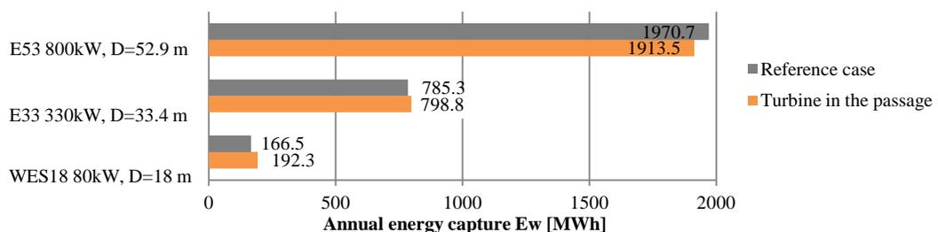
Figure 5: Annual energy produced by free-standing wind turbines and turbines in passages
