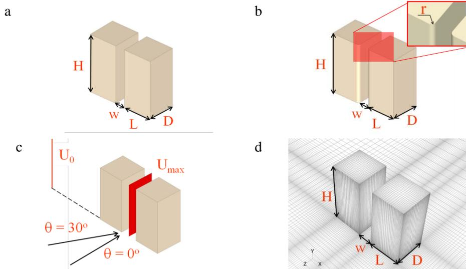
Figure 1: (a) Set-up overview. (b) Configuration with rounded edges ( $r = 5$  m). (c) Indication of considered wind directions and positions where  $U_{\max}$  and  $U_0$  are obtained. (d) View of the computational model and mesh.
