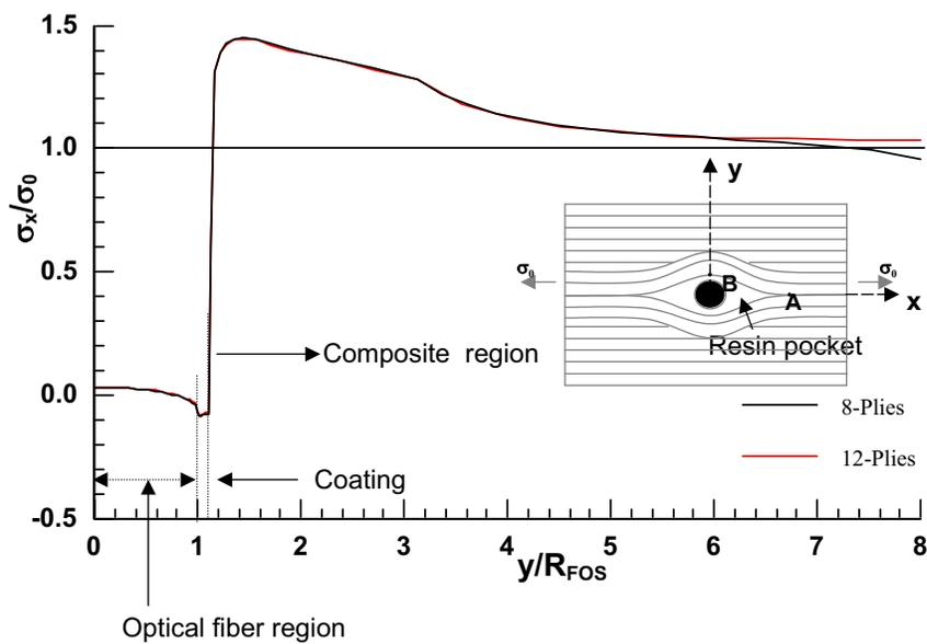
Figure 15 : Variation of  $\sigma_x$  along y-axis
